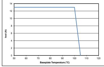
Figure 3: Maximum output current vs. base plate temperature (nominal input voltage).
