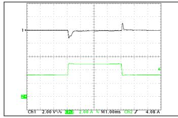
Figure 5: Output voltage response to step-change in load current (50%-75%-50% of Iout(max);  $dI/dt = 0.1 A/\mu s$ ). Load cap: 1  $\mu$ F ceramic capacitor. Ch 1: Vout, Ch 2: Iout (2A/div.)
