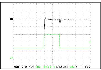
Figure 6: Output voltage response to step-change in input voltage (1000 V/ms). Load cap: 1  $\mu$ F ceramic capacitor. Ch 1: Vout, Ch 2: Vin.
