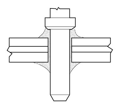
Figure F: Example of properly soldered pin joint
