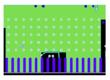
Figure G: Image of thermal via layout surrounding converter in test board
