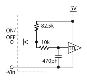
Figure B: Internal ON/OFF pin circuitry
