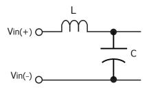
Figure D: Internal Input Filter Diagram (component values listed on specifications page).
