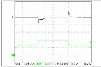
Figure 5: Output voltage response to step-change in load current (50%-75%-50% of lout(max); dI/dt = 0.1 A/µs). Load cap: 1 µF ceramic and 15 µF tantalum capacitors. Ch 1: Vout, Ch 2: lout (5A/div.)
