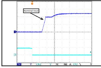
**Common Figure 1:** Typical startup waveform. Input voltage pre-applied, ON/ OFF Pin on Ch 2. See Note 3 for each voltage output.
